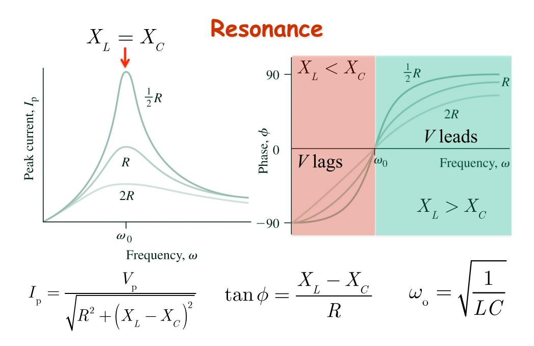
At resonance, Z = R, and  $\phi = 0$  (just like a DC circuit)
